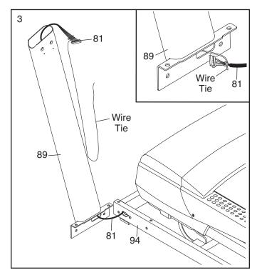
4. Hold the Left Upright (89) against the Base (94). Be careful not to pinch the Upright Wire (81). Insert two 3/8" x 1 1/4" Bolts (8) with two 3/8" Star Washers (13) and two 3/8" x 2 3/4" Bolts (7) into the Left Upright.
